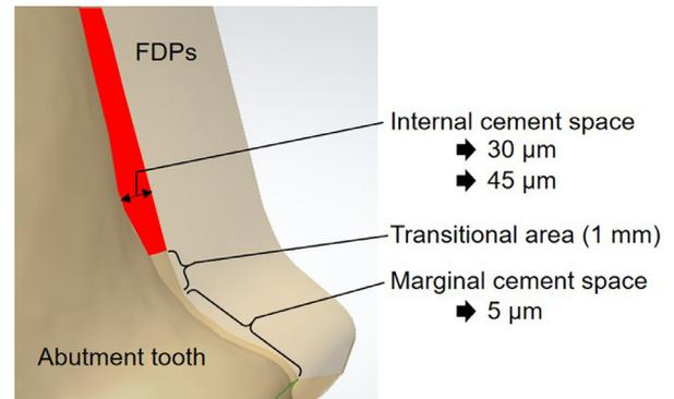
**Fig. 2.** Cement space used in each experimental group.
