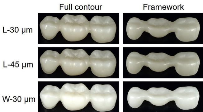
**Fig. 3.** FDPs fabricated in this study. Full contour (FC) and Framework (FW). Multi-layer structure (L) and Single-layer structure (W).
