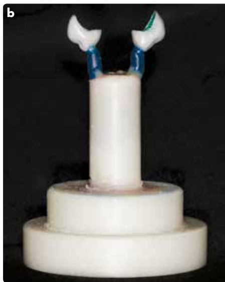
Figure 6b: Waxed up IPS e.max® (Ivoclar Vivadent, Liechtenstein) crowns ready for pressing
