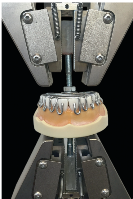
Supplemental Figure 3. Experimental design for measuring retention force of I-bar clasps engaging on teeth.
