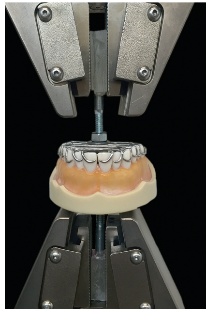
Supplemental Figure 2. Experimental design for measuring retention force of circumferential clasps engaging on teeth.
